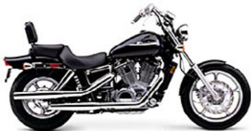
A two-wheeled motorcycle which consists of a full view engine, upright operator seating position with extended or pull back handlebars and forward mounted foot controls (for example: Suzuki Intruder, Harley Davidson FX series, Honda Shadow and Yamaha V-Star).
